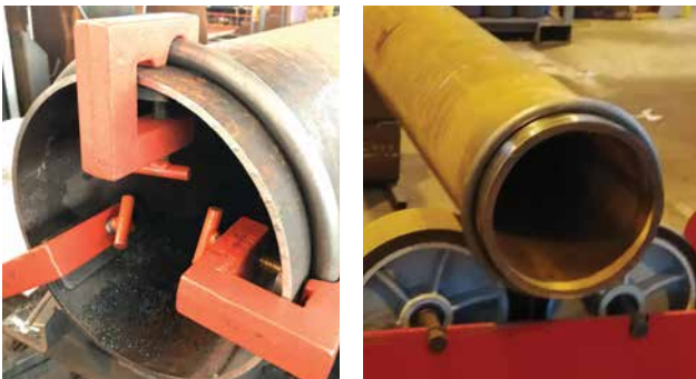
FIGURE 13: EXAMPLE OF WELD RING AND TUBE END PREPARATION
